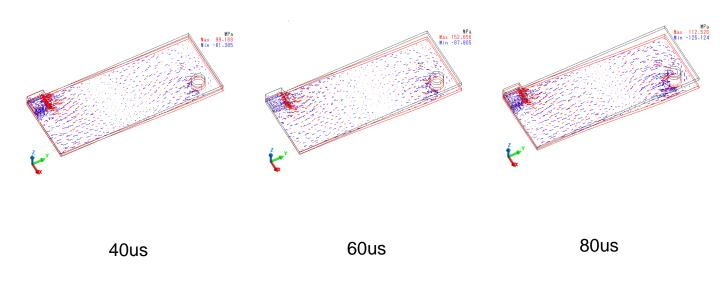
Large tensile stress is generated around the centrally mounted part in the longitudinal direction.
