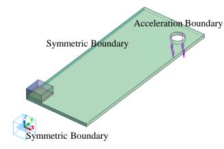
The model is a quarter-symmetric model of a substrate with a component mounted at the center. The symmetric face is set with a symmetric boundary condition (Fix). Acceleration boundary is set to the inner surface of the hole located at the corner of the substrate. See the next slides for more information.
