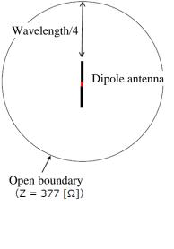
**The open boundary** is a boundary condition where electromagnetic waves do not reflect. The open boundary is provided by using the plane wave's wave impedance of free space, which has a value of  $377 \Omega$  by default.
