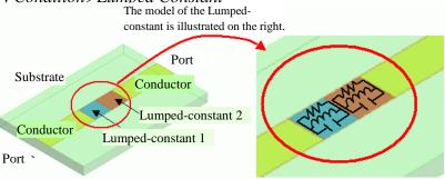
Set the lumped-constant boundary to the portion between two conductors.
