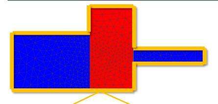
The finite element method requires all the outermost faces of a model to be set with boundary conditions.
