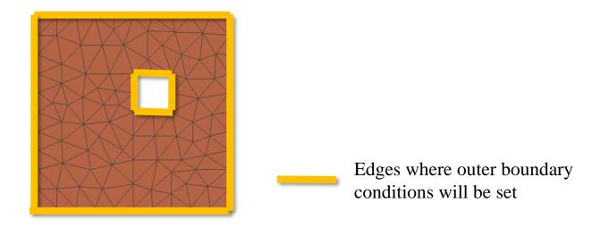
If any boundary condition is not set to the circumference of the inner hole, the outer boundary condition will be set thereto.
